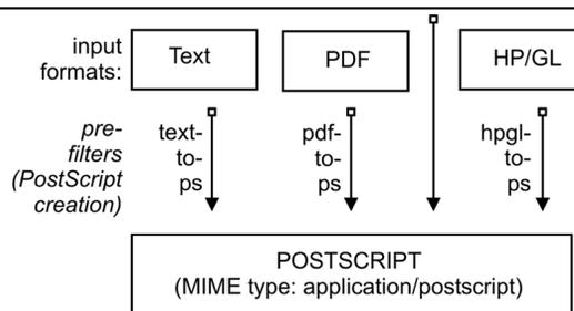
**Figure 21.4.** Prefiltering in CUPS to Form PostScript.
