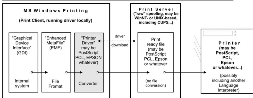
Figure 21.13. Print Driver Execution on the Client.
