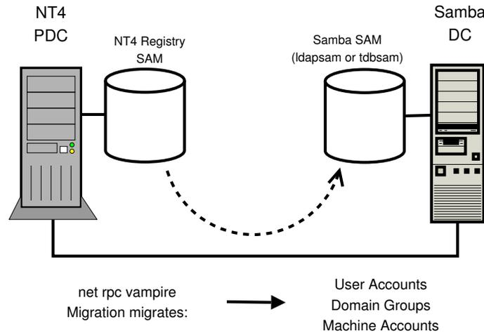
**Figure 9.1.** Schematic Explaining the net rpc vampire Process
