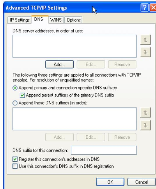
**Figure 8.4.** DNS Configuration.
