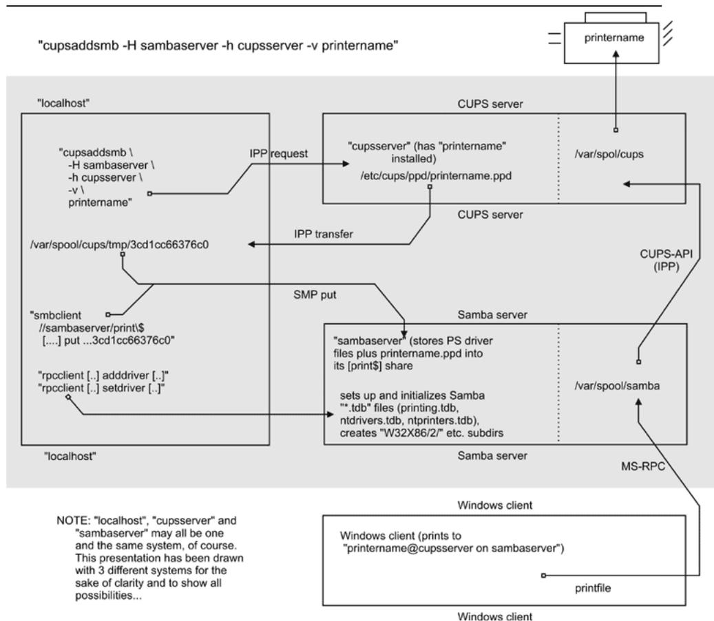
Figure 21.16. cupsaddsmb Flowchart.
