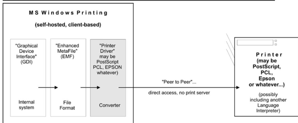
Figure 21.1. Windows Printing to a Local Printer.
